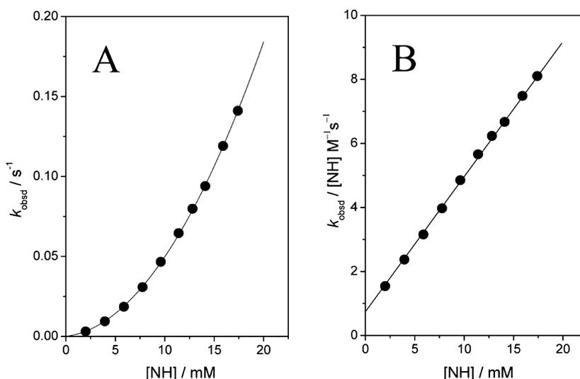
Figure 1. Plots of  $k_{\text{obsd}}$  vs [NH] (A) and  $k_{\text{obsd}}/[\text{NH}]$  vs [NH] (B) for the reaction of  $\beta$ -nitrostyrene (**1g**) with piperidine in MeCN at  $25.0 \pm 0.1$  °C.
