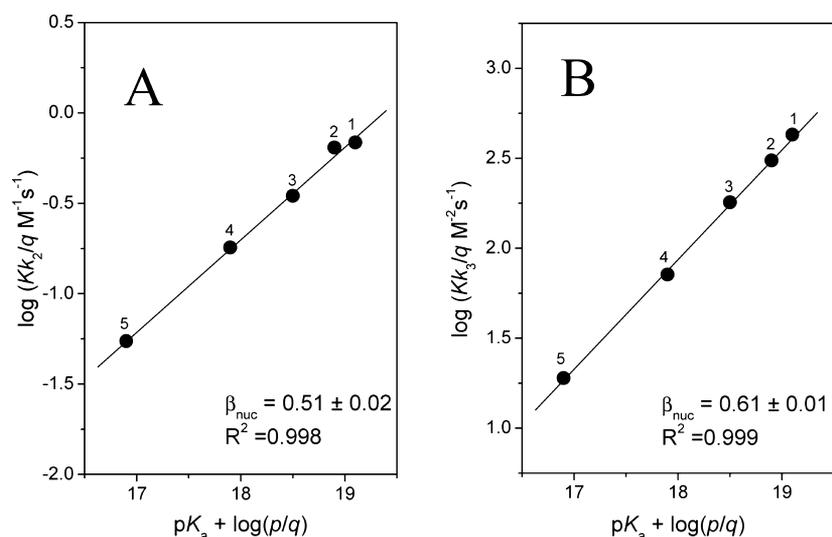
**Figure 2.** Bronsted-type plots for the reactions of  $\beta$ -nitrostyrene (**1g**) with cyclic secondary amines in MeCN at  $25.0 \pm 0.1$  °C.  $\log Kk_2$  vs  $pK_a$  (A);  $\log Kk_3$  vs  $pK_a$  (B). The identity of the points is given in Table 1.
