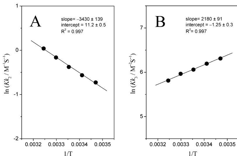
Figure 4. Arrhenius plots for the reactions of  $\beta$ -nitrostyrene (**1g**) with piperidine in MeCN.  $Kk_2$  (A) and  $Kk_3$  (B).
